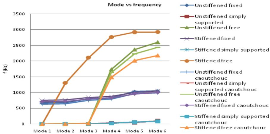
Fig. 11. Representation of natural frequency with respect to modes for various test specimens.
