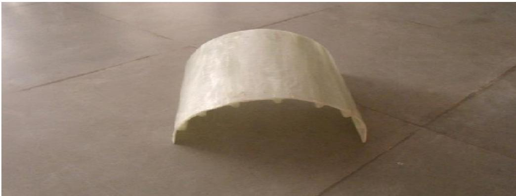
**Fig. 2.** Fabricated specimen with longitudinal stiffener.
