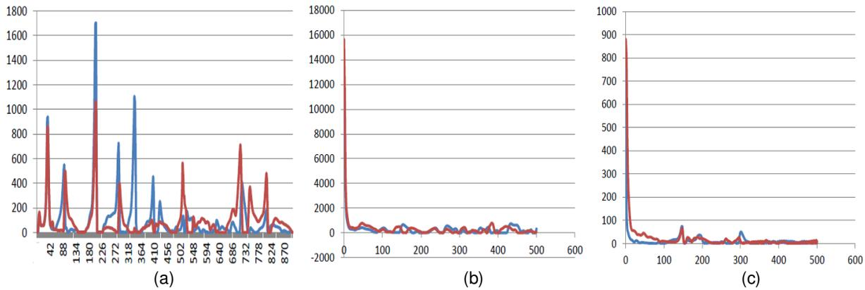
**Fig. 8.** Response curves of stiffened (a) free (b) simply supported (c) fixed shells having frequency in Hz as x-axis and amplitude along y-axis.
