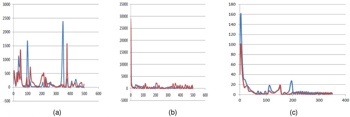
**Fig. 9.** Response curves of unstiffened (a) free (b) simply supported (c) fixed shells with 5% caoutchouc having frequency in Hz as x-axis and amplitude along y-axis.
