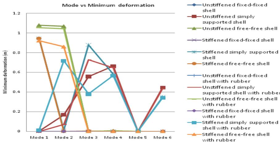
Fig. 13. Representation of minimum deformation with respect to modes for various test specimens.
