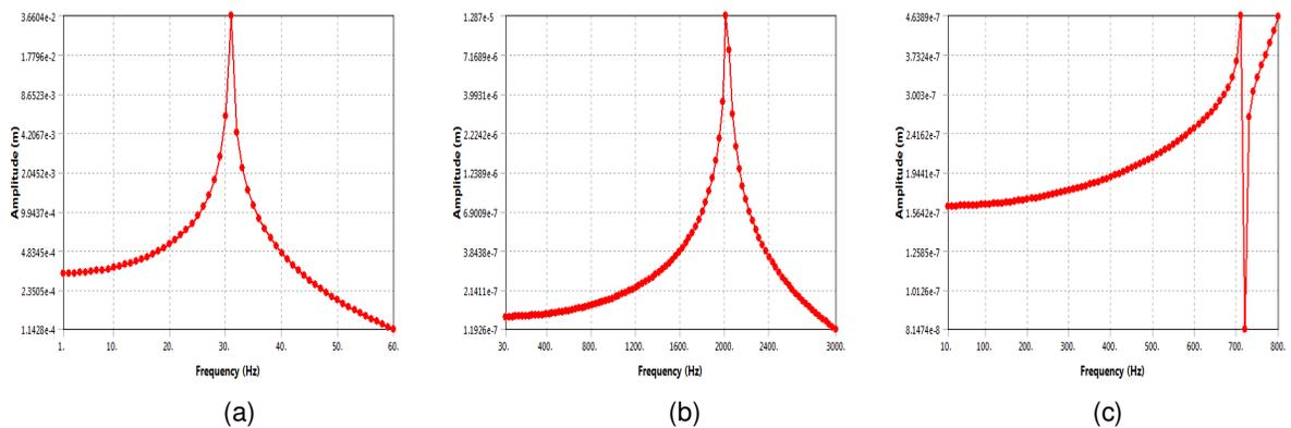
**Fig. 17.** Response curves of Stiffened (a) free (b) simply supported (c) fixed shells with 5% caoutchouc having frequency in Hz as x-axis and amplitude along y-axis.
