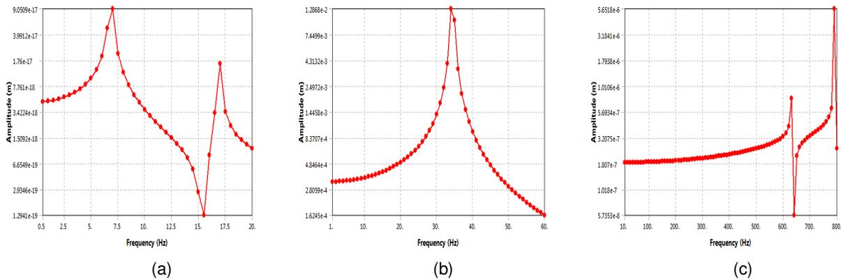
**Fig.16.** Response curves of unstiffened (a) free (b) simply supported (c) fixed shells with 5% caoutchouc having frequency in Hz as x-axis and amplitude in m as y-axis.
