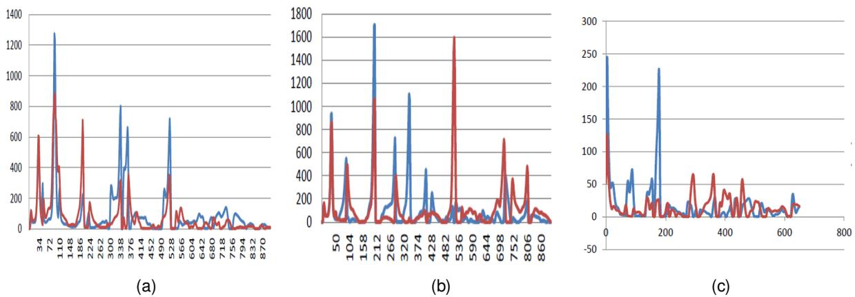
**Fig. 7.** Response curves of unstiffened (a) free (b) simply supported (c) fixed shells having frequency in Hz as x-axis and amplitude along y-axis.
