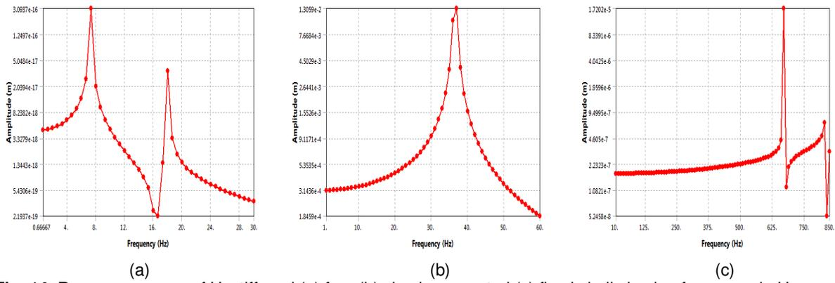
**Fig. 14.** Response curves of Unstiffened (a) free (b) simply supported (c) fixed shells having frequency in Hz as x-axis and amplitude along y-axis.
