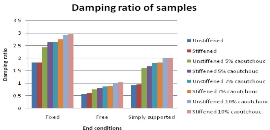
Fig. 19. Comparison of damping ratio (numerical) for various shells with different end conditions.
