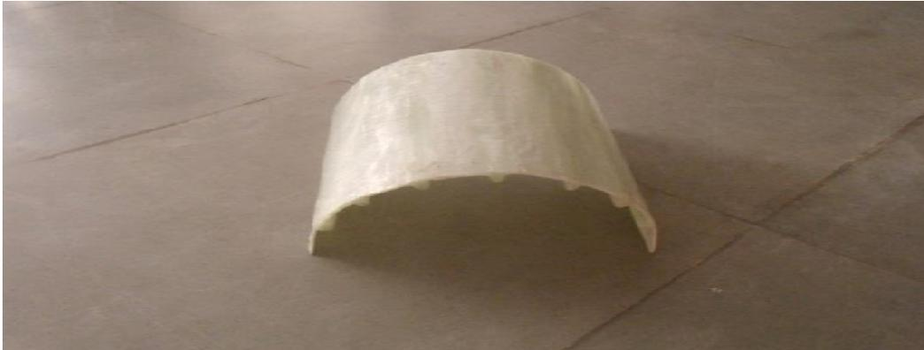
**Fig. 2.** Fabricated specimen with longitudinal stiffener.
