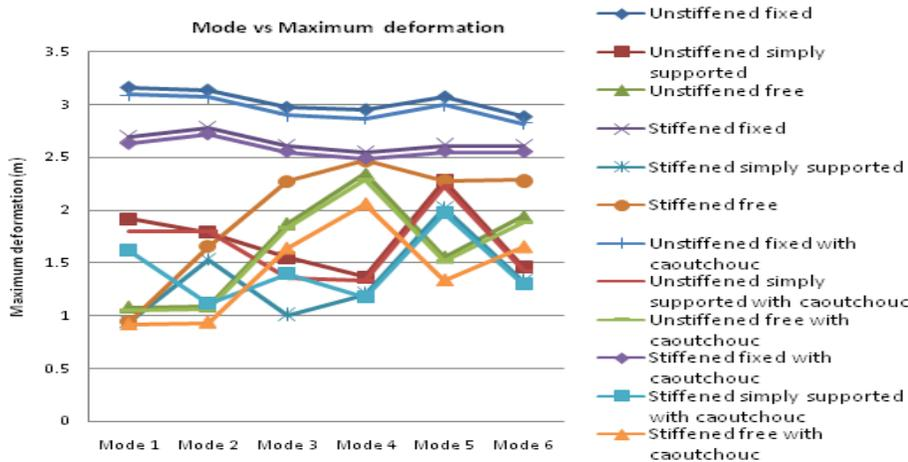
Fig. 12. Representation of maximum deformation with respect to modes for various test specimens.
