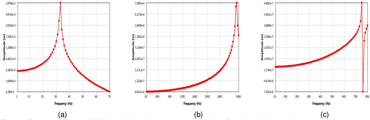
**Fig. 15.** Response curves of Stiffened (a) free (b) simply supported (c) fixed shells having frequency in Hz as x-axis and amplitude along y-axis.
