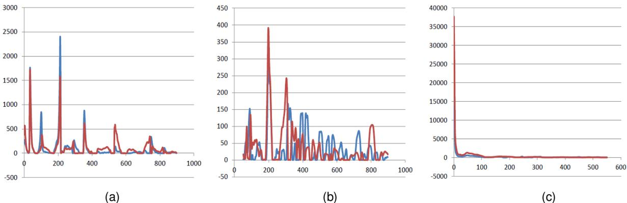
**Fig. 10.** Response curves of stiffened (a) free (b) simply supported (c) fixed shells with 5% caoutchouc having frequency in Hz as x-axis and amplitude y-axis.
