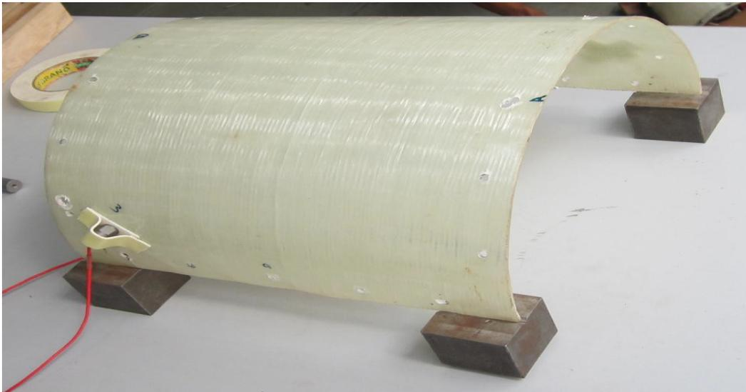
**Fig. 5.** Simply supported end condition.
