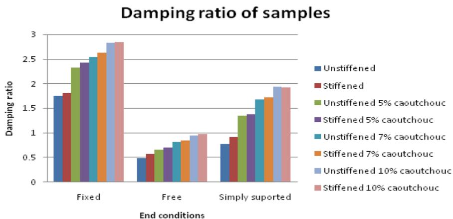
Fig. 18. Comparison of damping ratio (experimental) for various shells with different end conditions.
